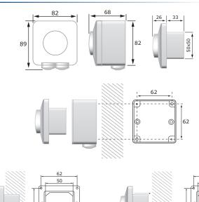
Speed controller for EC motors
